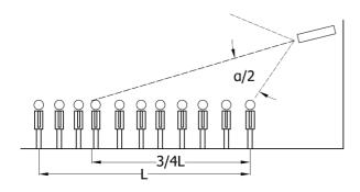
The opening of polar pattern have to be also sufficient to cover horizontally the entire area where there are listeners. The opening of polar pattern is configurable by the interface in the central unit.
