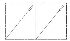
In stereo application every area have to be covered by two projectors (left and right).
