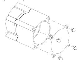
Disassembling the rear cover find a numeration label, the numbers have to coincide with the numeration in the speakon 8 pole male connector.
