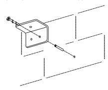
4) Now you can put the speaker temporary in the supports and make some little hole for the screws (2 or 3 millimetres could be sufficient, it is related to the screws used).
